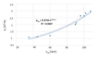
Fig. 15. Equation of the function of the expected values of charging air pressure
