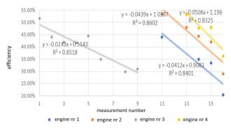
Fig. 12. Trends in compressor efficiency reduction for four engines in selected operational periods
