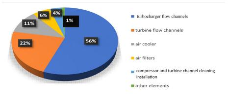
Fig. 3. Contribution of contaminants and sludge to the effect on engine performance
