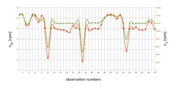
Fig. 9. The main engine speed and turbocharger rotor speed runs as a function of observation numbers
