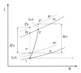
Fig. 6. The air compression process in enthalpy-entropy coordinates
