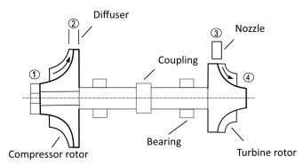
Fig. 5. Diagram of a turbocharger rotor unit with control plane numbers
