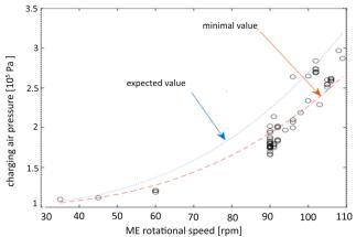
Fig. 14. A function describing the relationship between the expected values of air charge pressure  $p_{2ex}$  and a function describing the minimum acceptable values of air charge pressure  $p_{2min}$  in relation to the main engine shaft speed (ME)
